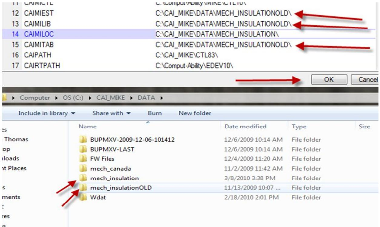
Also update then “Start Tables” logical name, to point to the new INI file, just like the Target in the new MIKE 10 shortcut. This will allow access to the new database, within the Tables module. Then Click “OK” to close the window.
